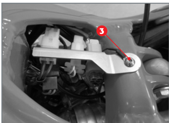
Connectors support version 125cc - 250cc - 300cc.
