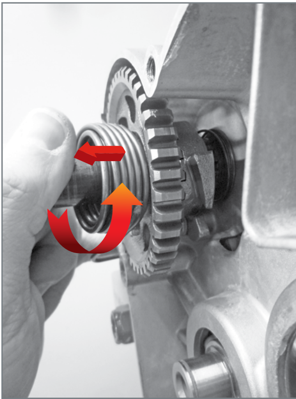
Extraction of shaft from crankcase.
