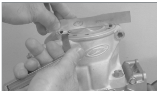
Case where the piston pushes the plate causing cylinder/plate contact to be lost
