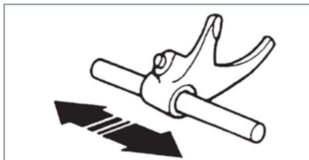
Check fork sliding on pin.
