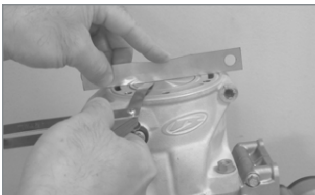
Case where the plate and piston do not touch: check distance between plate and piston.
