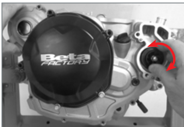
Application of complete inner clutch cover on right crankcase.
