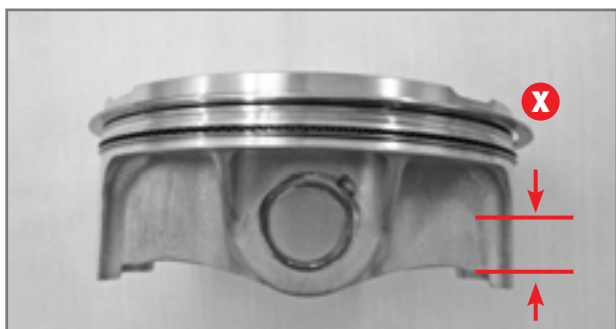
Position to measure the outside diameter of the piston.
