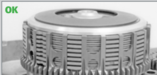
Detail of correct fitting of the spring washer.
