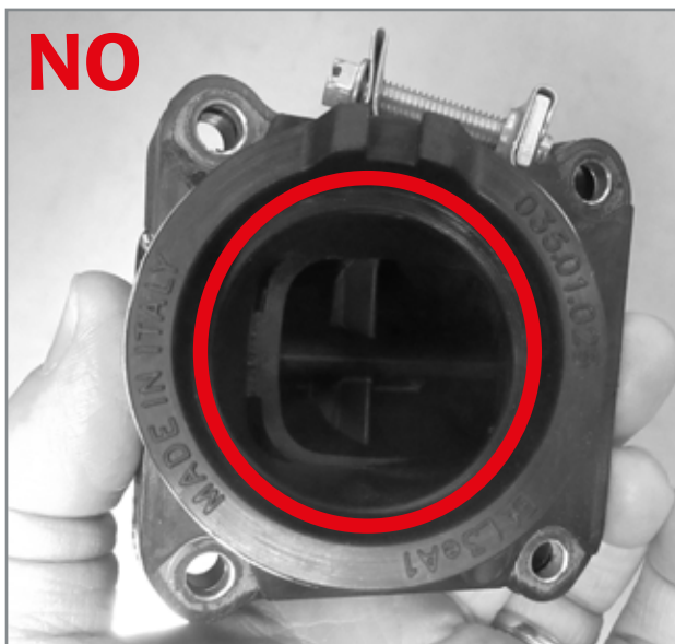
Disassembly of central wedges. The extraction of only one is shown in figure.
