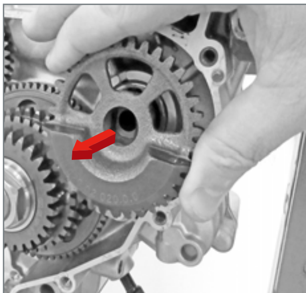
Extraction of countershaft.
