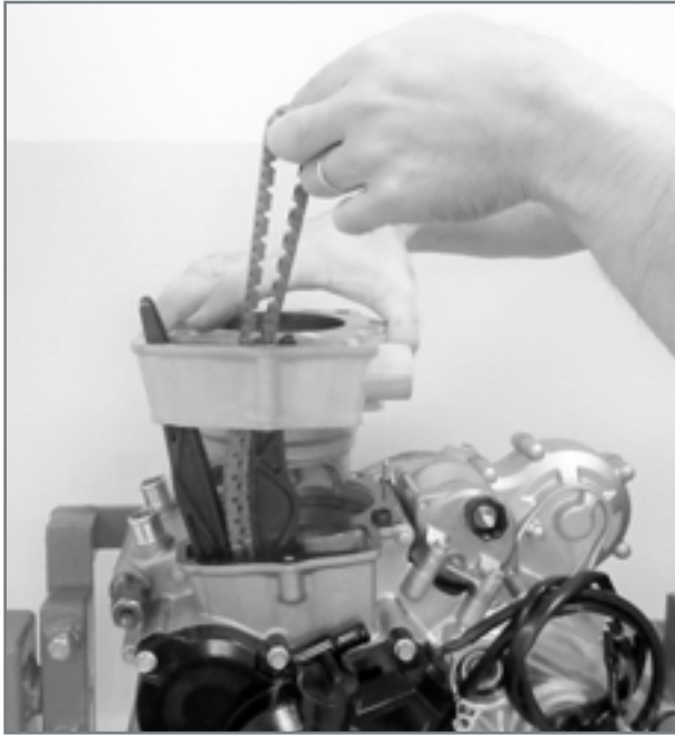
Passing the chain through the cylinder.
