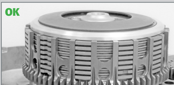
Detail of correct fitting of the spring washer.
