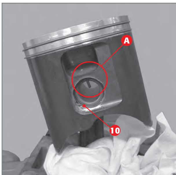
Removal of piston circlip.
