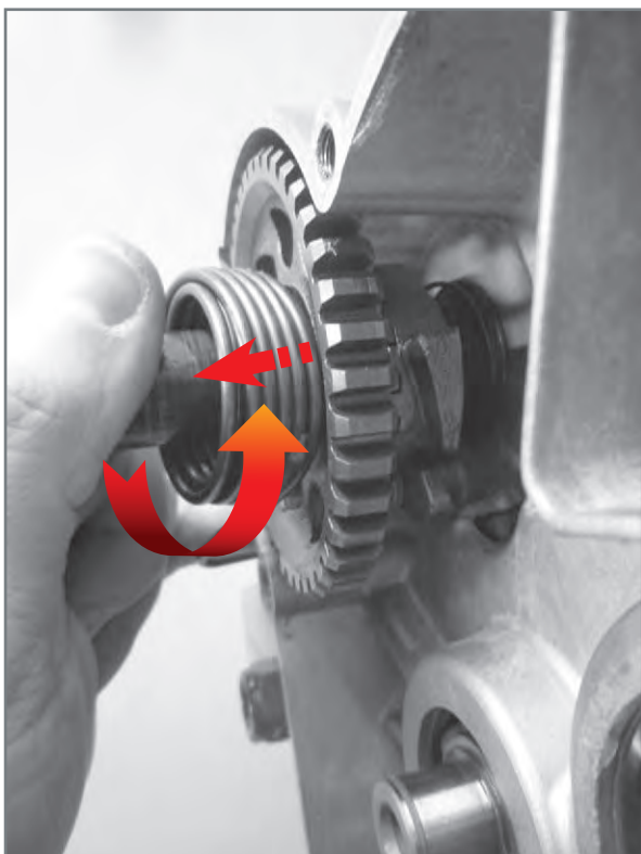
Extraction of shaft from crankcase.
