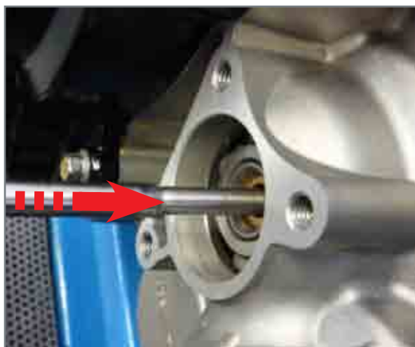
Insertion of clutch rod.
