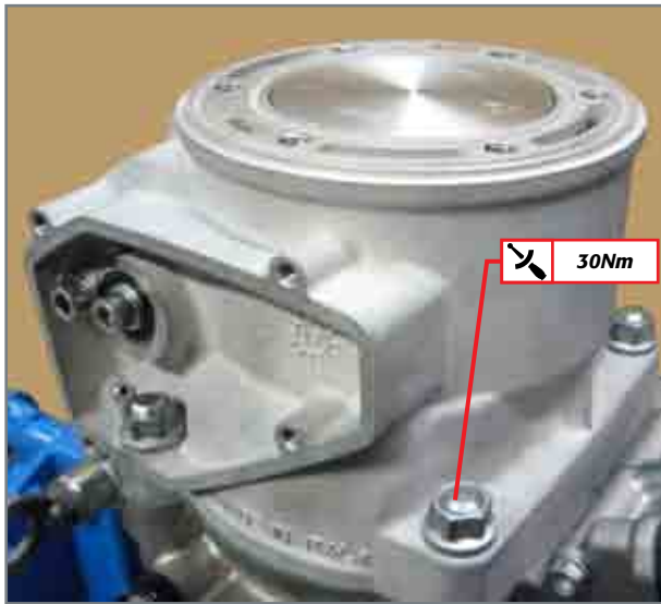
Fastening of cylinder nuts.
