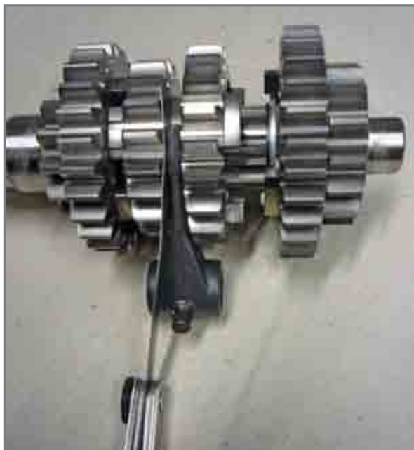
Check of wear of forks and gearwheels.
