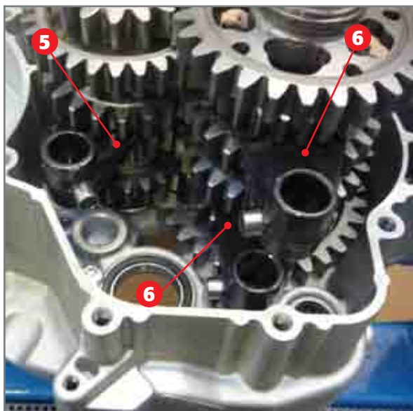
Application of forks to gearwheels.
