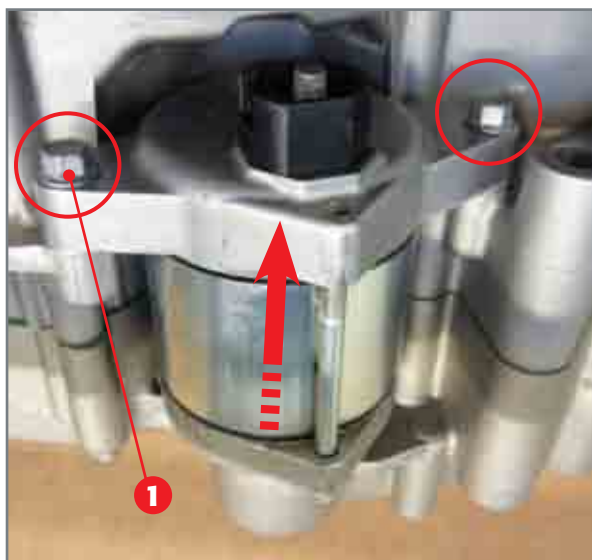
Removal of start motor.
