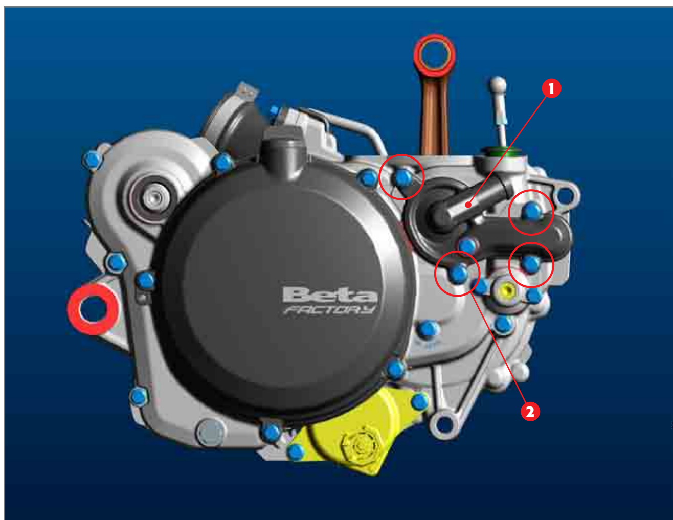
Coolant liquid pump cover screws.
