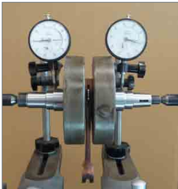
Deflection/Off-centring of crankshaft.
