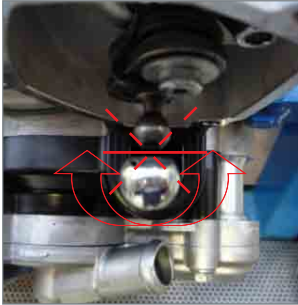
Check of control rod rotation.
