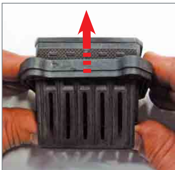
Disassembly of reed valve body.
