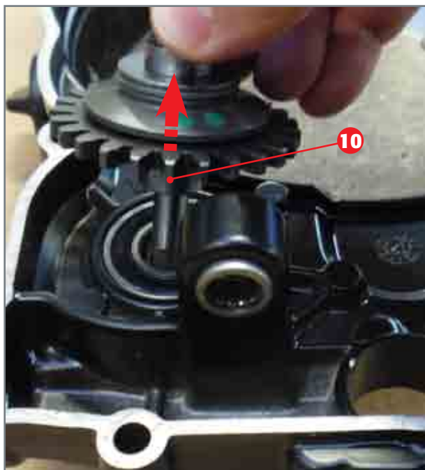
Extraction of centrifugal unit.
