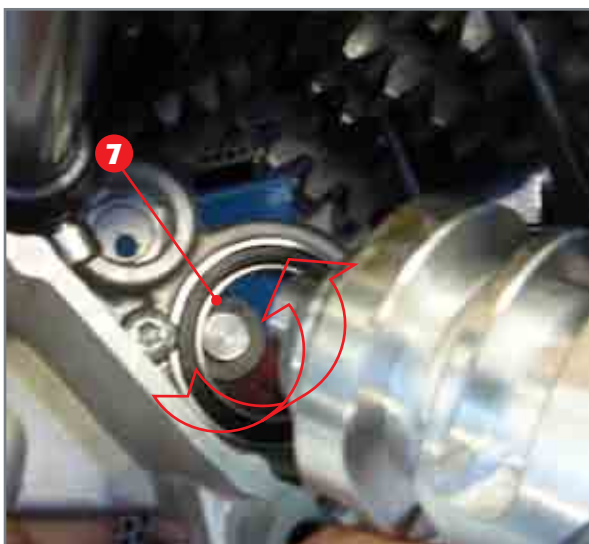
Insertion of desmodromic device in specific bearing. Note the rotation of the stop lever.
