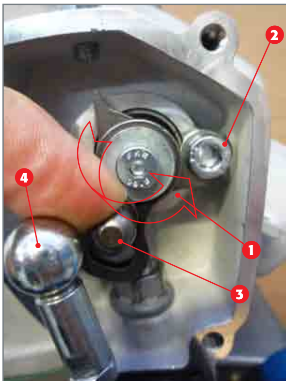
Positioning of valve control.
