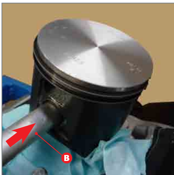
Removal of pin bolt.
