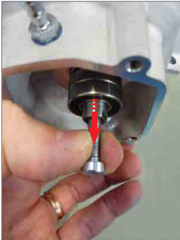
Extraction of booster.
