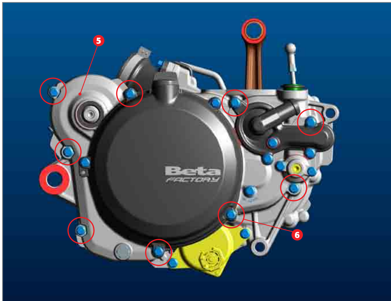
Inner clutch cover screws.
