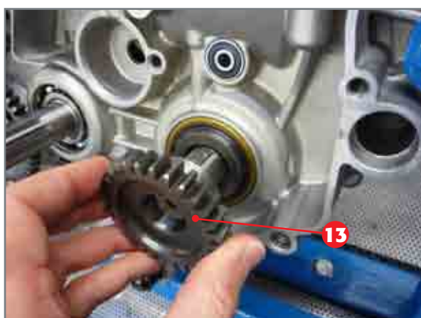
Removal of main gear.
