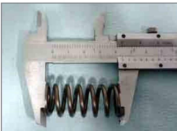
Clutch spring length measurement.
