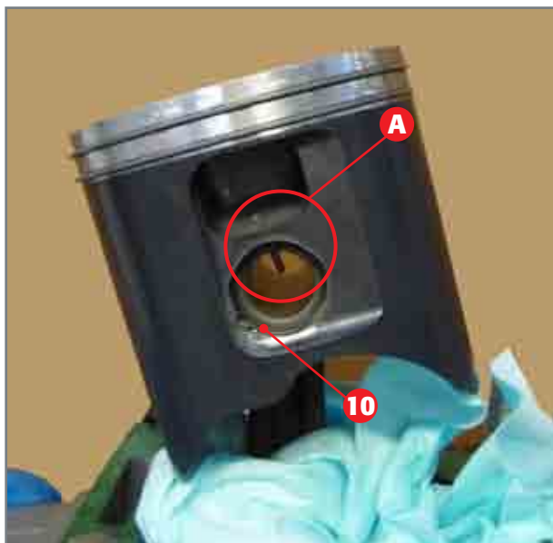
Removal of piston circlip.
