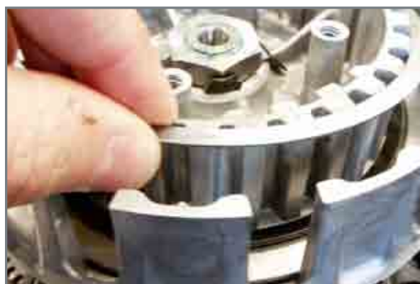
Removal of disc spring assembly.
