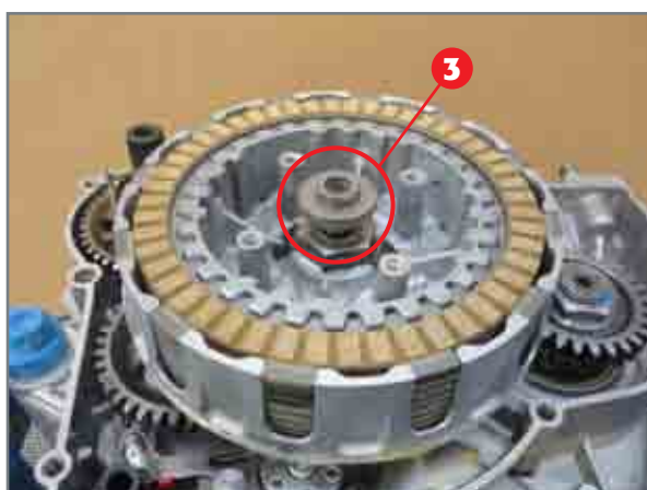
Pressure plate unit 3 and clutch disc pack.
