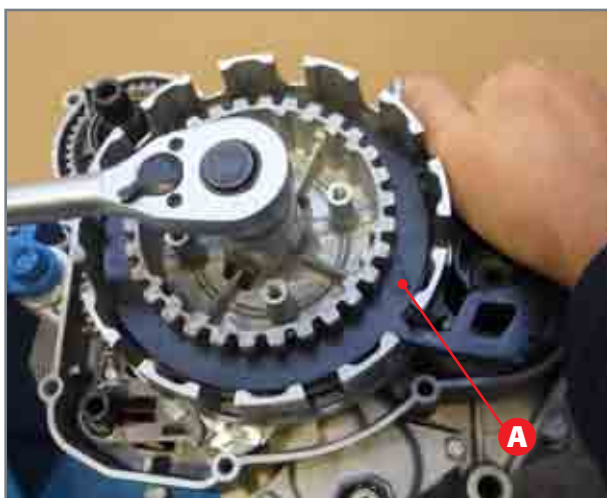
Removal of clutch drum nut with relevant tool A.
