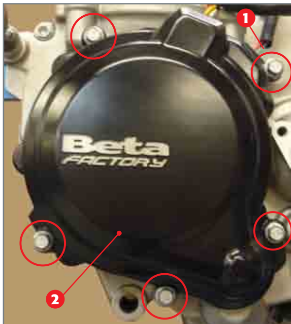
Fixing screws 1 of flywheel cover 2.
