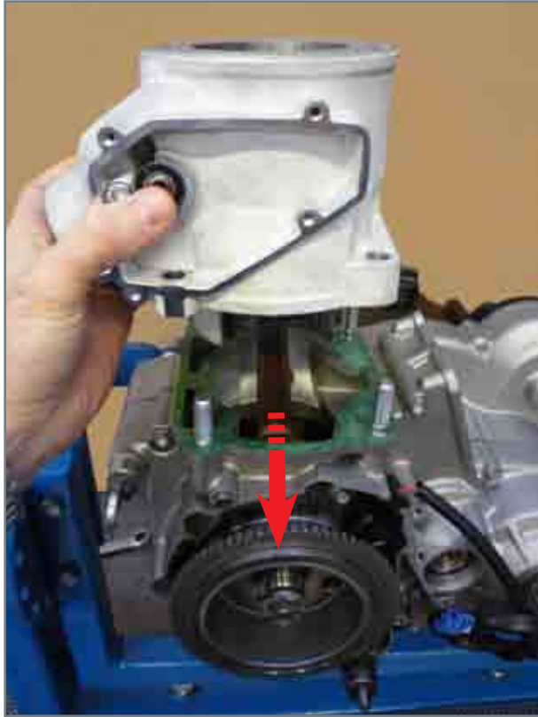
Coupling of cylinder to piston and crankcase-
