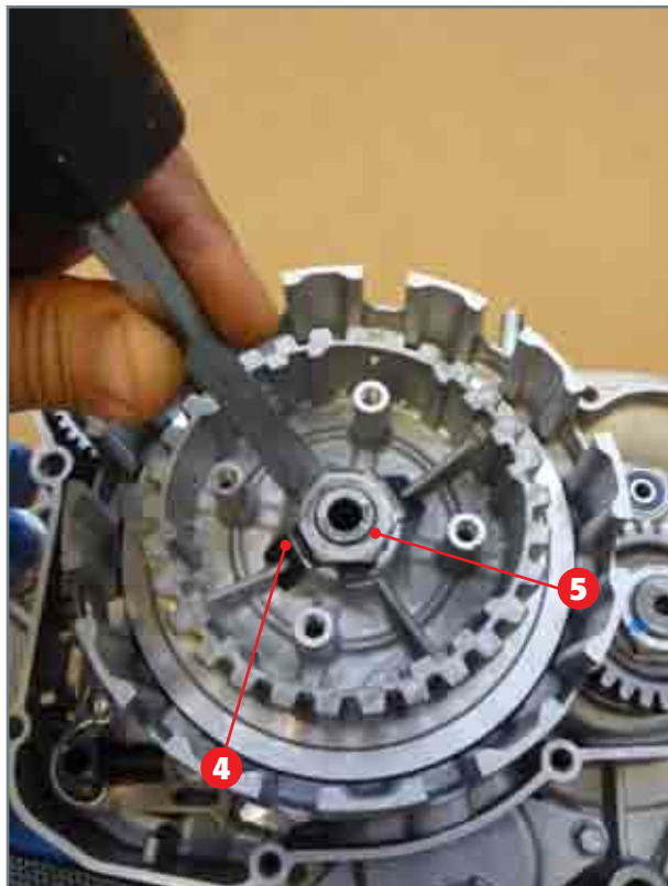
Opening of the safety washer with chisel.
