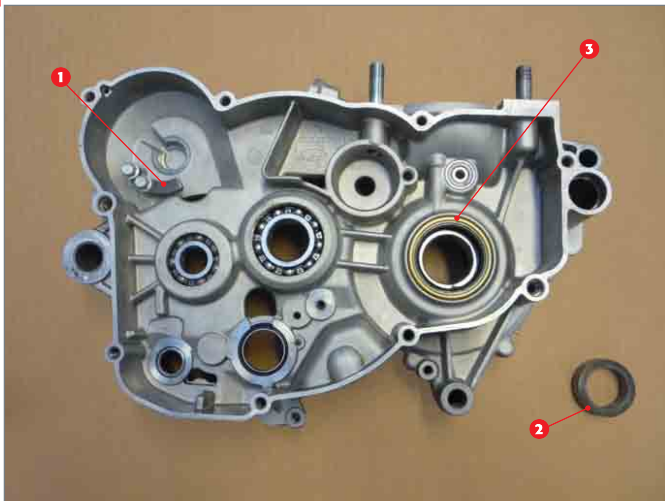
Kickstart ramp 1), crankshaft spacer 2) (and relative O-ring), oil seal 3).
