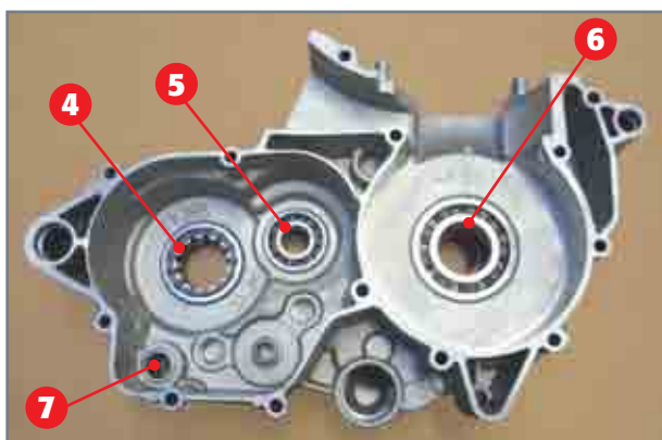
Removal of left crankcase half bearings.
