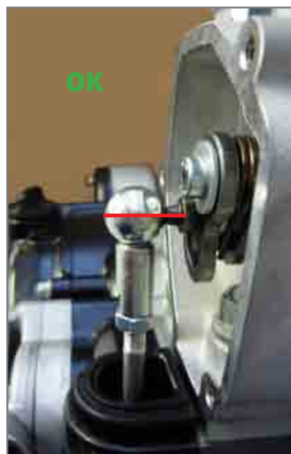
Correct position of the control rod seat.
