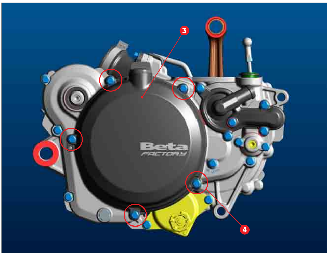
Outer clutch cover screws.
