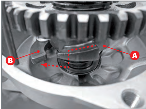
Positioning of sleeve A below ramp B.
