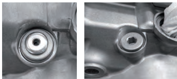
Rivet on pressure re- gulator. Pressure regulator.
