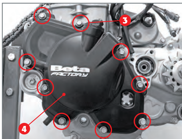
Fixing screws C of ignition cover D.
