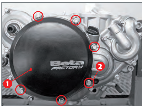
Outer clutch cover 1 and respective screws 2.
