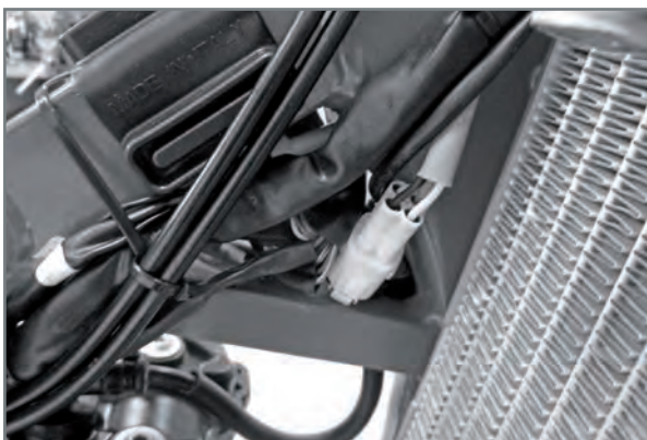
Electric connectors in the recess (carburettor versions).
