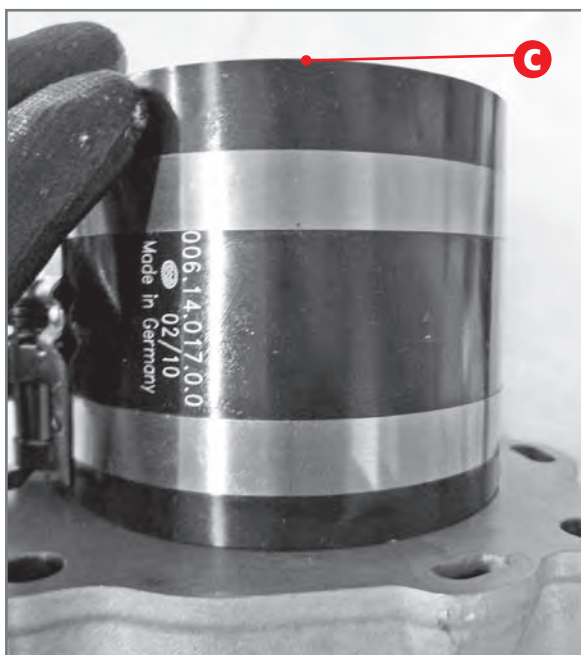
Application of the complete piston band on cylinder.
