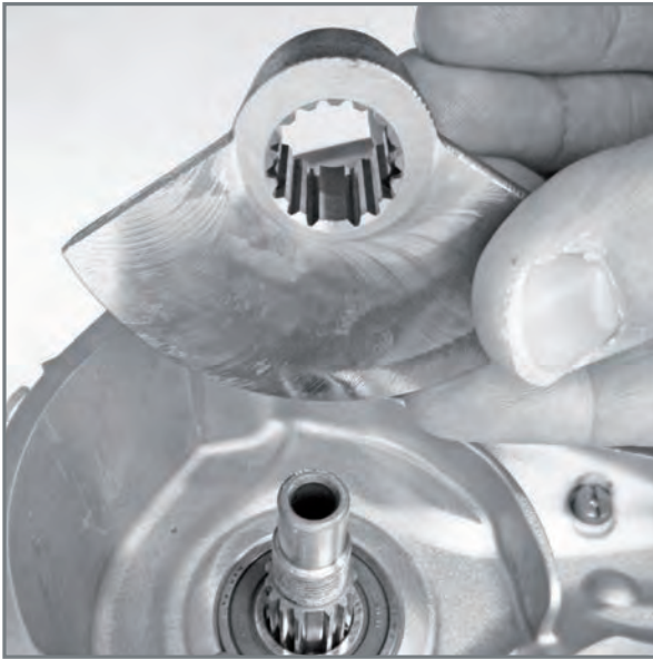
Coupling counterweight to countershaft.
