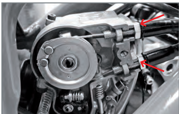
Carburettor version gas cables.
