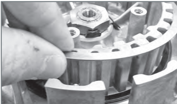
Removal of disc spring assembly.
