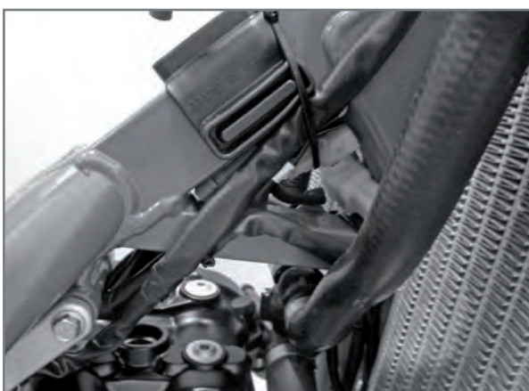
Electric connectors in the recess (injection versions)..
