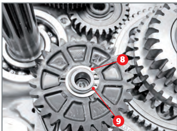
Coupling pump control wheel.
