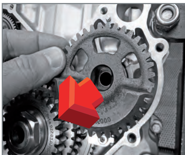
Extraction of countershaft.
