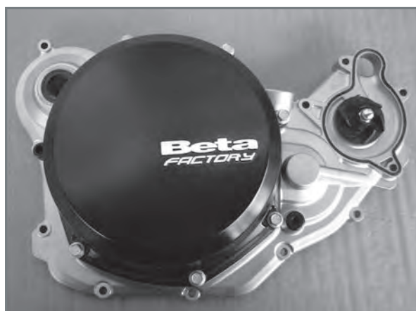
Complete internal clutch cove of water pump.
