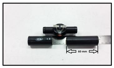
Cut out 35mm from the lower cooling hose to allow room for the thermoswitch assembly making sure that one of the hoses is roughly 60mm in length as shown.
