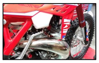
Reinstall the fuel tank, fill the radiator with coolant making sure the coolant system has been bled.
