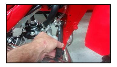
Remove the lower radiator hose and clamps. You will install the thermoswitch into this hose later.
