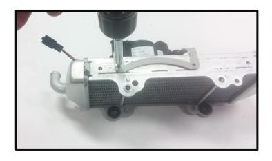
Install the fan bracket to the radiator using the three self-tapping screws.
