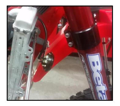
After all of the coolant has been drained, remove the right side radiator by removing the fuel tank, then disconnecting the hoses and removing the two bolts holding the radiator onto the frame.
