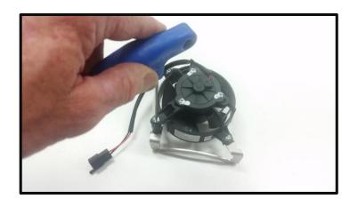
Install the fan motor using the three nutclips and screws provided as shown in the photo
