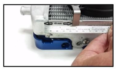
Adjust the bracket so that there is 45mm from the edge of the radiator to the bracket as shown.
