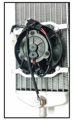
Using a screw gun, use the four self-tapping screws to mount the fan brackets to the radiator.
