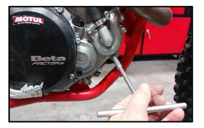
When the engine is cold, remove the radiator cap and drain the coolant into a clean container.
