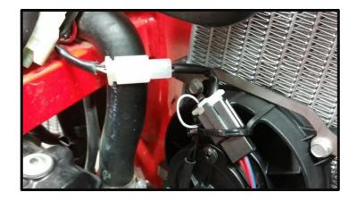
Re install the radiator, hoses, and coolant making sure the cooling system is bled. Plug the fan kit into the open connector on the motorcycles stock wire loom.
