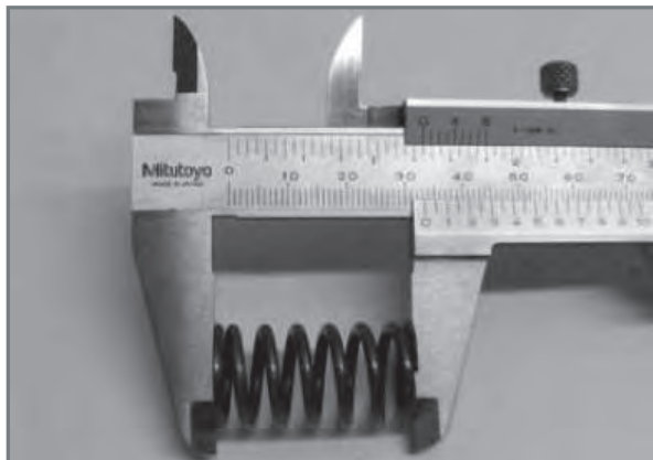
Measuring the length of the clutch springs.
