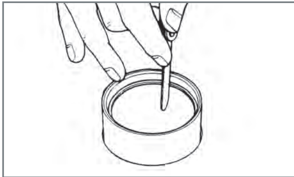
First verification of the piston rings.
