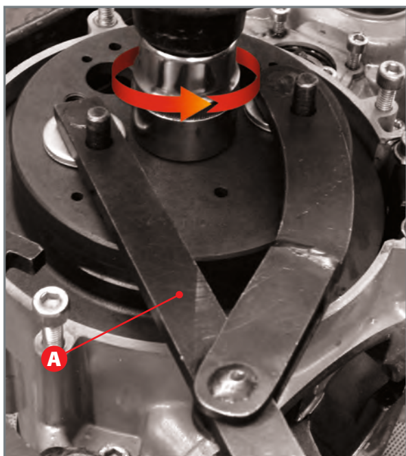
Removal of flywheel nut.
