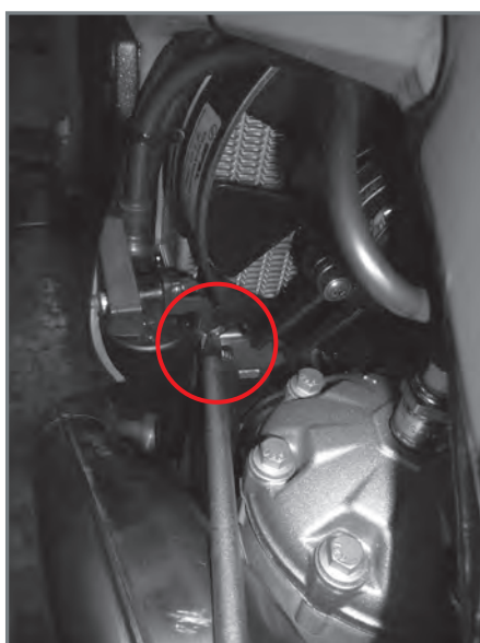
Reassembling the coil and support.
